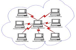
Figure 2: Single piconet ad hoc network.
